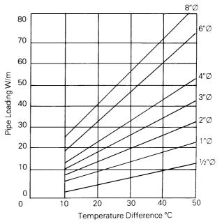
The above graph is based upon lin thermal insulation similar to mineral wool with K factor  $0.05W/m^{\circ}C$ .
