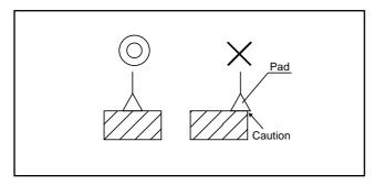
When conveying large surface area plates with multipads, the most important thing is the well balanced positioning of pads, and care should be taken to prevent pads from protruding beyond the plate.
