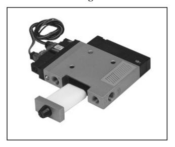
An all in one vacuum generator, silencer, suction filter incorporating an on/off air supply valve. This valve switches the air supply and therefore vacuum on or off via the in-built solenoid. Additionally the unit has a vacuum release (blow-off) valve. This valve switches a positive pressure to quickly release the object being picked. An integral flow control valve provides adjustment to the rate of flow of air used to release the object.
