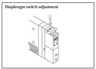
There is a slotted adjuster on top of the vacuum switch for setting actuation vacuum pressure levels.
