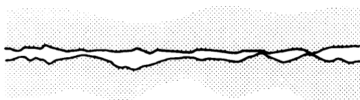
Figure 1 Contacting surfaces magnified
