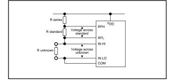
The ratiometric technique is used for resistance measurements. The unknown resistance is placed in series with a known resistor and current is passed through the pair. The voltage developed across the unknown resistor is applied to the input (INHI, INLO). The voltage across the known resistor is applied to the reference inputs RFH and RFL. If the unknown equals the standard, the display will read 1000.
