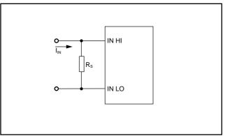
Current measurement requires a shunt resistor  $(R_{\rm s})$  to convert the input current into a 200mV input voltage as shown above. This shunt can also be used to adjust the meter scale factor.
