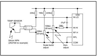
The sensing transistor has a temperature coefficient around -2mV/°C. To calibrate, place sensor in iced water (0°C) and adjust zero for a 000.0 reading. Then place sensor in boiling water (+100°C) and adjust scale factor for a 100.0 reading. The sensor would normally be built into a protective housing.
