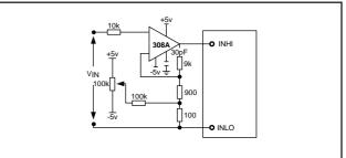
An operational amplifier is used to measure full scale voltages less than 199.9mV. Note that the auto-zero circuitry within the module cannot compensate for the op amp offset or voltage drift.
