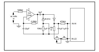
The module can only measure dc. The diagram above shows an ac to dc converter circuit that can be used to measure ac. Alternatively to measure true RMS the following ICs would be suitable. Please refer to the Semiconductors-Analogue/Linear ICs section of the **RS** Catalogue. AD636JH **RS** stock no. 302-665, AD736JN **RS** stock no. 658-328.
