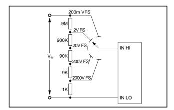
Multirange voltmeters are easy to implement using a rotary or push-button switch system as shown. It is necessary to also switch the decimal point. This can easily be accomplished by connecting the appropriate D1 to D3 terminals with a rotary switch to  $V_{\text{DD}}$ .
