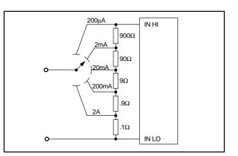
Multirange current meters can be produced using a rotary or push-button switch system as shown.
