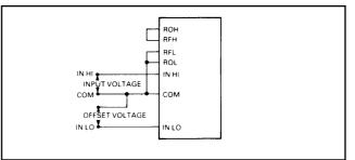
If a zero display is required when the input voltage level is not zero, the offset voltage should be connected between INLO and COM while the input voltage is connected between COM and INHI.
