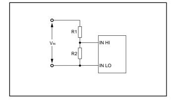
To measure voltages greater than 200mV an input attenuator is required, as shown above. This attenuator can also be used to adjust the meter scale factor. R1 and R2 should be accurate and stable. Good metal film resistors meet these requirements.
