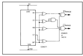
Connections for generating the over- and under-range signals for use in auto-ranging applications.
