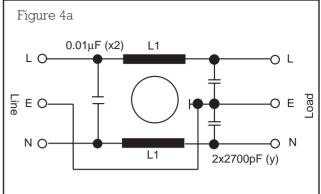
Simplest transient protection filter using double wound flux cancelling inductors  ${\rm Ll},\,{\rm Ll}$
