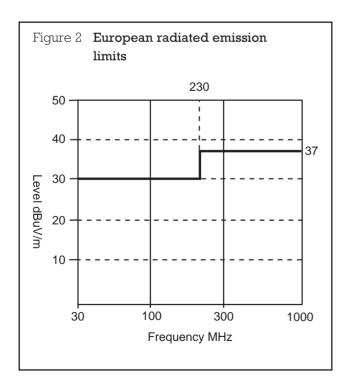
In order to ensure continuity of measurements, the conducted emissions are measured with a standard receiver with defined time constraints, impedance and attenuators against a standard mains supply line impedance stabilisation network, the radiated measurements are made using standard receivers with calibrated antennae against a specified ground plane in an open site of set minimum size and distances.
